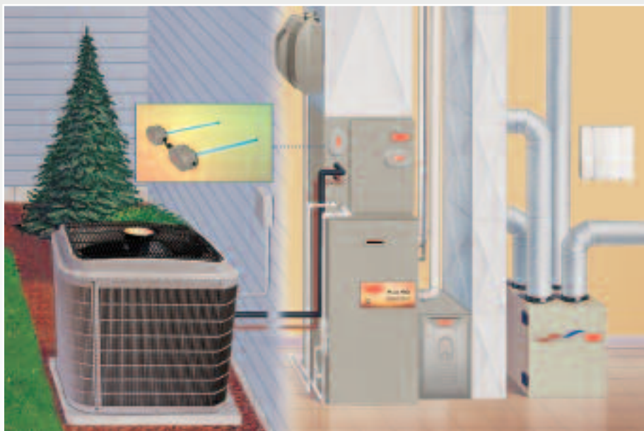
Air Conditioner and Gas Furnace System
